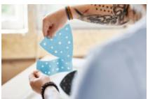
**Triple sanding:** The new Granat Delta 200 abrasive can be used three times: The tip can simply be torn off at the perforation, turned and reused. This reduces abrasive consumption, saves costs and conserves resources - for sustainable work in the Festool system.
