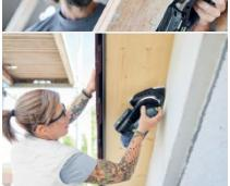
**Independent working:** Practical and independent working without a mobile dust extractor. No matter where, the dust collection bag for the DTSC 200 offers maximum freedom of movement when sanding, without a cumbersome suction hose.
